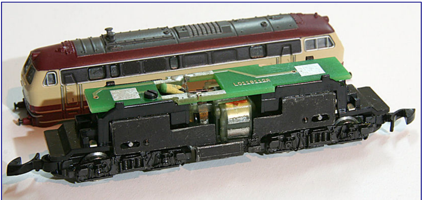
After removing the housing, the analogue locomotive appears as shown in this picture: The printed circuit board is held in place by four lugs and a screw (left).
