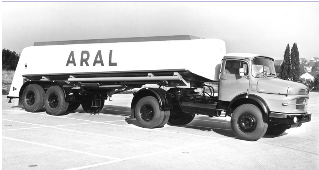
As demand increased, so did the amount of fuel to be transported. Tankers therefore also made use of the weight permitted by the registration regulations. In 1965, articulated lorries, like this Mercedes short bonnet with Aral semi-trailer, had long been commonplace. Photo: Historisches Archiv BP/Aral
