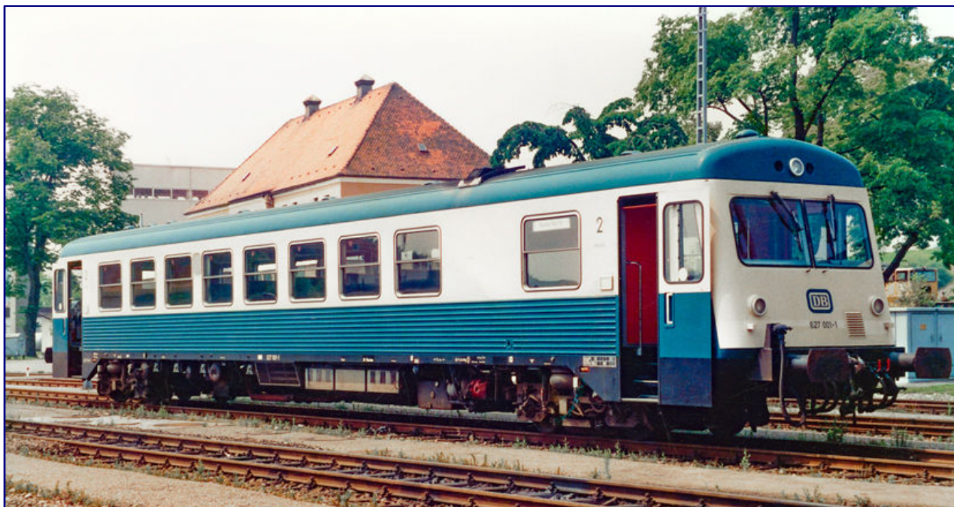
This photograph taken on 13 July 1985 in Kempten (Allgäu) shows the 627 001-1 of the German Federal Railways in operating condition, which the planned SMZ model is also intended to reproduce. The railcar was converted to regular train and buffing facilities the year before. Photo: Malte Werning
