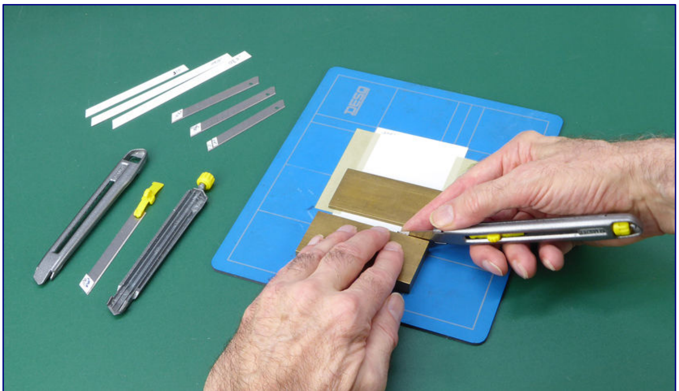
This is how the cutting process shown on page 11 works in reality. On the left are the dismantlable blade holders and the snap-off blades with different spacers for different sized strips.
