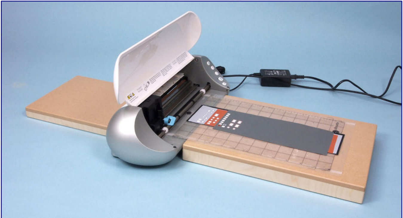
The self-made lay-on plates on the small Silhouette CNC cutting plotter make it possible to make changes to the foil package during a break in the cutting process.
