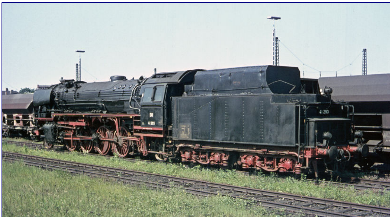
Photo above: Unit tenders 2'2' T 32 were not that rare on the German Federal Railway. Also 03 054 (Bw Köln-Deutzerfeld) is shown in April 1955 in Oberhausen Hbf. Photo: Reinhard Todt, Eisenbahnstiftung
