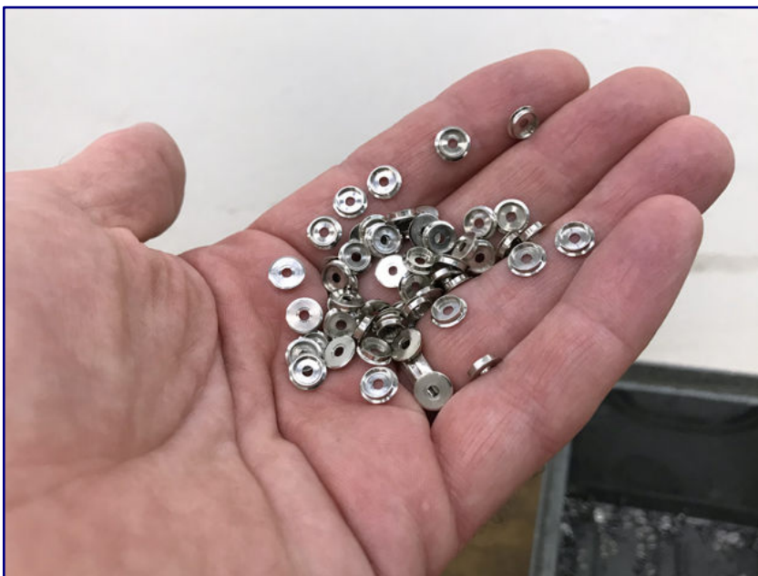
With open eyes during the tour, we discover turned parts for Z gauge wheels on the lathes of the Märklin factory in Göppingen.
