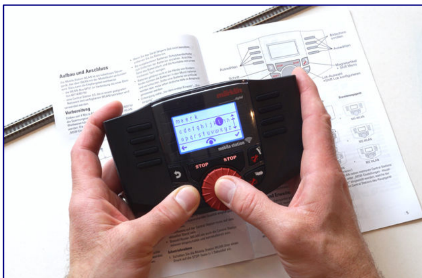
The unit is connected to the WLAN of the receiver box via the menu selection. It is then necessary to enter a password that is stored in the instructions.
