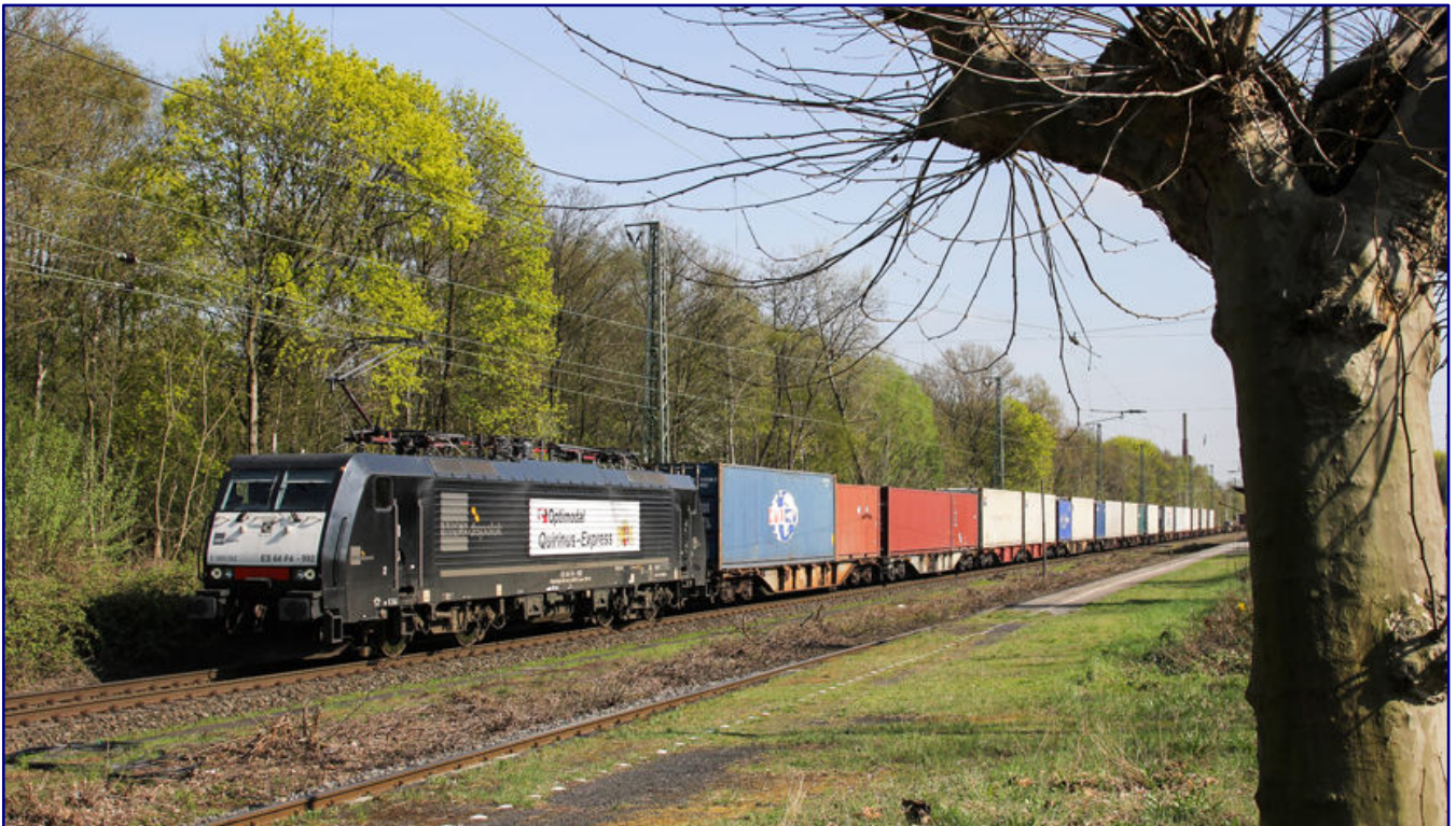
189 092-0 (ES 64 F4-992 from MRCE) passes through Dinslaken station on 6 April 2011 with a container train from Dortmund to Rotterdam. In second place behind the locomotive is an Sgns type wagon, presumably from the AAE fleet. Photo: Joachim Bügel, Eisenbahnstiftung
