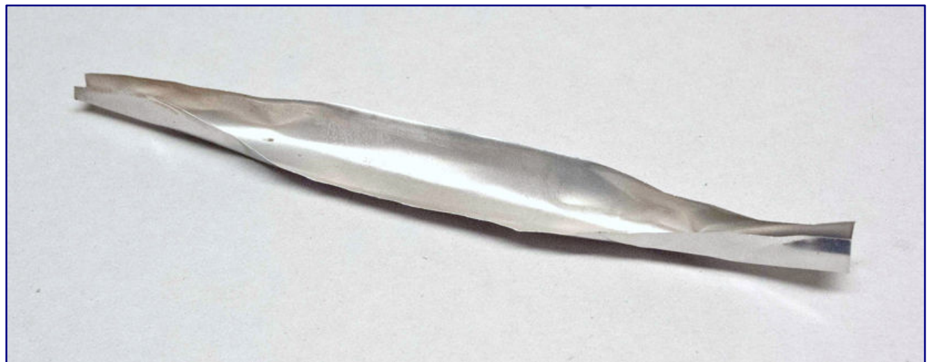
Inconspicuous, but valuable: self-made dumping tool made of aluminium sheet for spreading ballast and small chippings.
