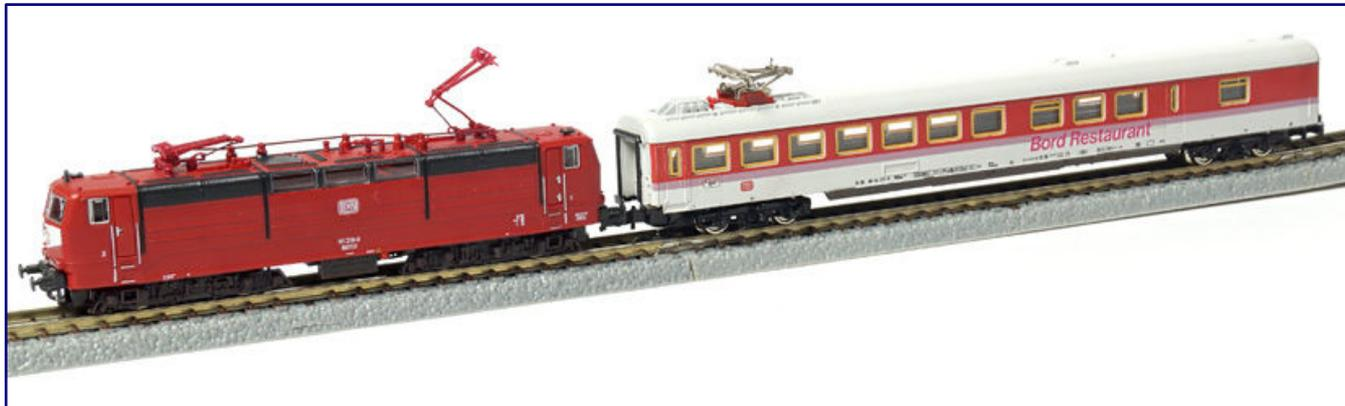
The class 181<sup>2</sup> from Rokuhan demonstrated how a single-arm pantograph SBS 67 should look to scale, and, thus, also justified requests for bodies for Märklin models. The additional shortcoming that Märklin's SBS 65 counterpart cannot be laid flat is particularly disturbing on the dining cars.
