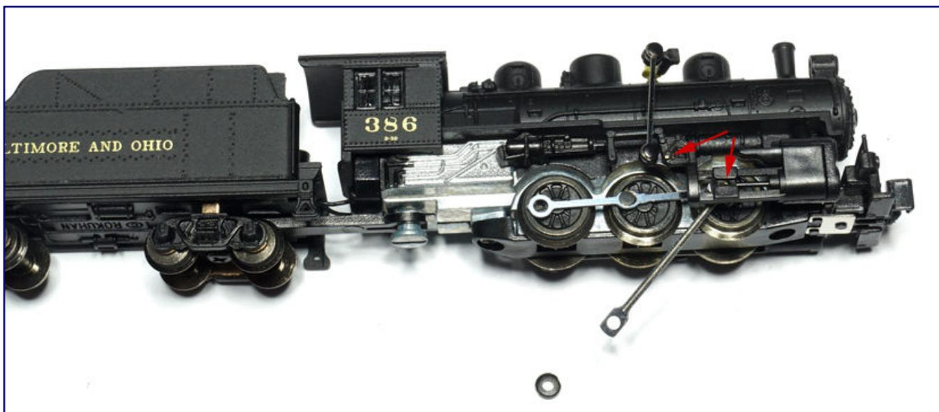
Right at the start of the first test drive, the pin of the counter crank on the drive axle fell out. The washer (bottom of photo) was inserted between the drive rod and coupling rod. Reassembling the control unit, which quickly disassembles completely, becomes a game of patience, especially since the retaining bolts marked with arrows have to be reinserted from the inside! There is an urgent need for a durable and operationally stable solution from the factory!
