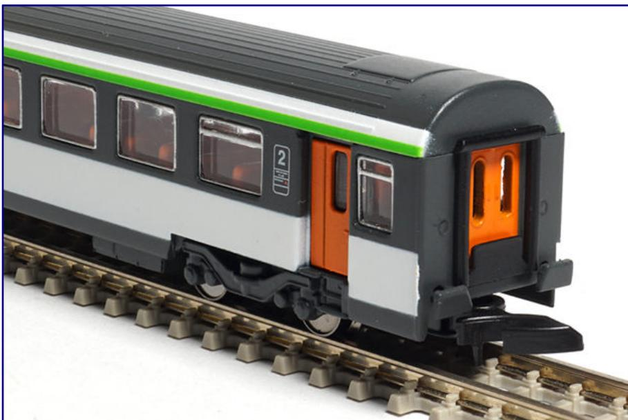
The carriage ends are almost exemplary: We find transparent inserts in the transition doors; the transition plate is distinctly set off and the oversized buffers are an important prototypical feature. The only things that remain on the wish list are the red taillights and the prototype's slightly curved waistband including the upper contrast band.
