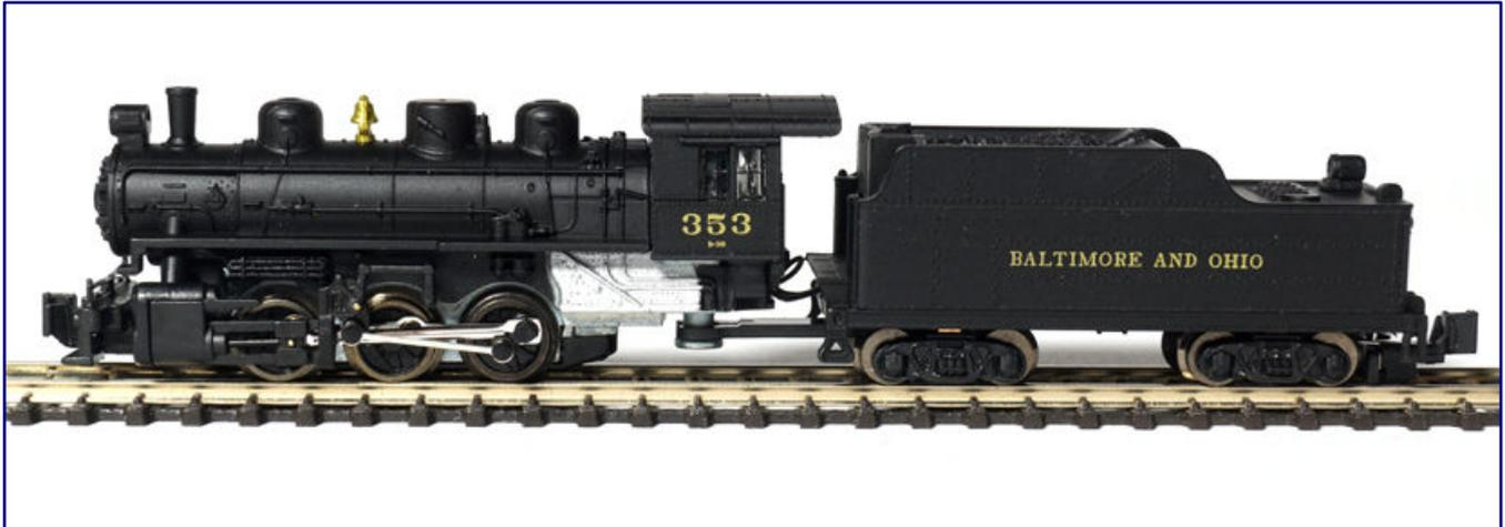
The second locomotive in our test bears the road number 353 (T040-2) and is shown here from its stoker side. Its linkage parts were checked and secured in good time before another failure could have occurred.
