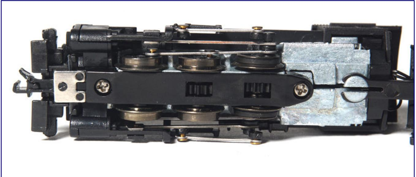
Looking from below, we discover two gear wheels that are not covered and can therefore collect dust fluff over time. There is no sign of current being drawn from the coupling wheels.
