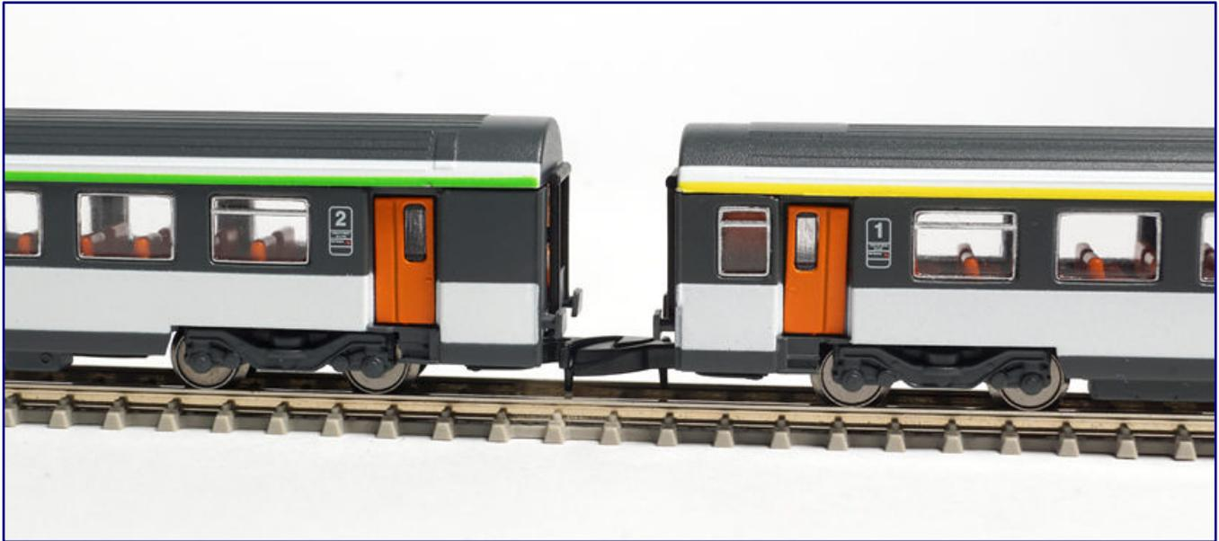
A decisive weak point of the new wagons is the far too great of a distance between the couplers, which is very annoying. Possible solutions could be close couplers or fixed coupling rods, but this needs to be tested at home on the installed radii and counter curves before the wagons are converted for use on the layout.
