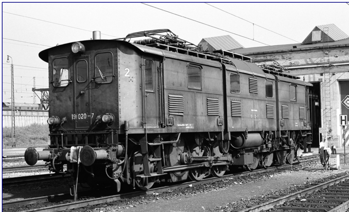
On 2 October 1971, 191 020-7 allows a good view of its running gear in the Munich East depot. The ladder, which was suspended transversely above the buffer beam, had long been seen on locomotives of this class. Photo: Burkhard Wollny, Eisenbahnstiftung
