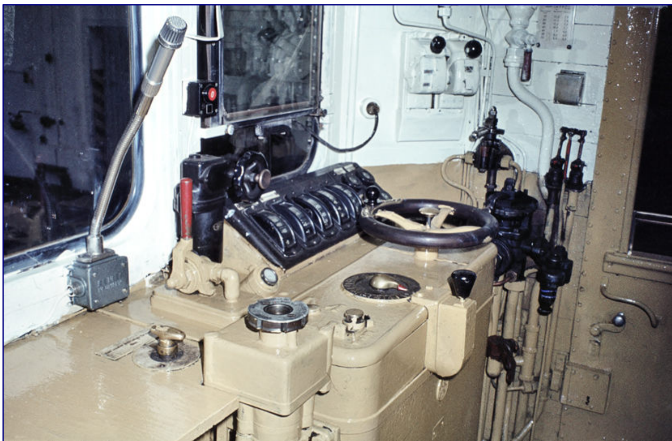
Interior view of the driver's cab of an E 91 0 , taken in March 1974 in Munich East. Like other old construction machines, this rod locomotive was also operated standing up. Photo: Walter Abriel, Eisenbahnstiftung
