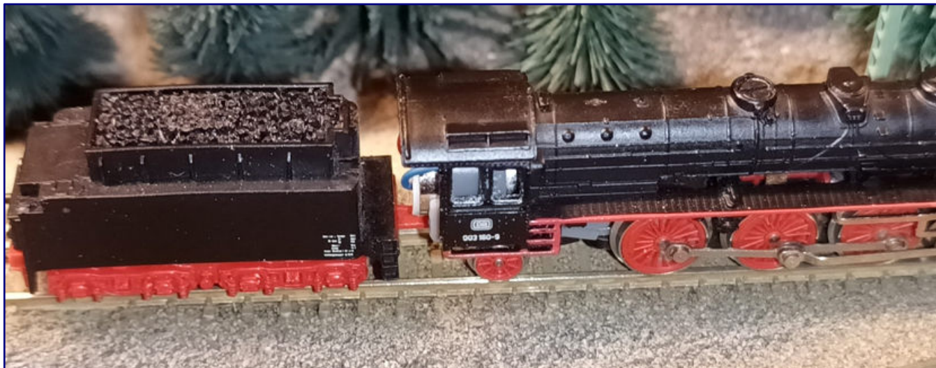
This is what the new motor mount with the 0812S bell-type armature motor looks like when installed without any further camouflage measures. Photo: Z-Otti | Hans-Jörg Ottinger
