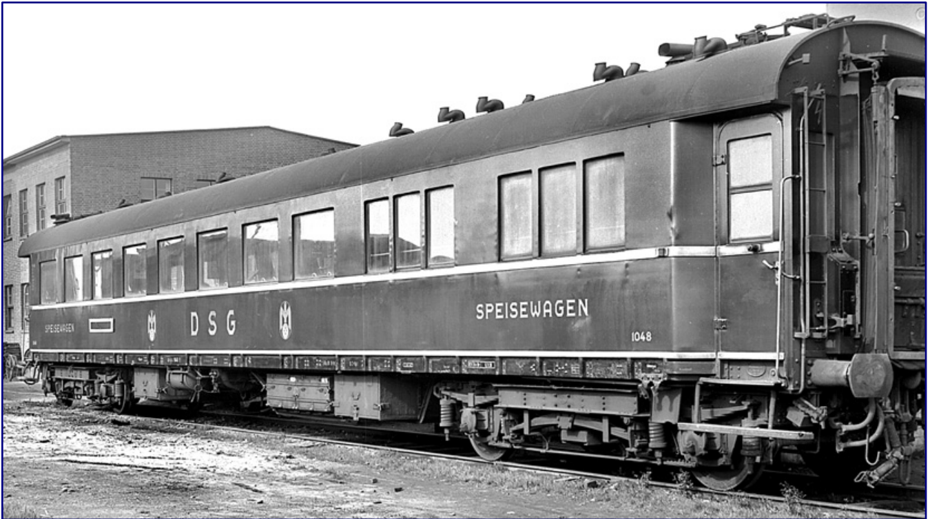
The DSG dining car 1048 photographed in 1956 is a WR4ü(e)-28 and thus belongs to the 1928 design. However, the rivets of the outer panels were recessed and flush-fitted on the dining cars. The preserved car is equipped with "Görlitz II heavy" type bogies. Photo: Engels | Eisenbahnstiftung
