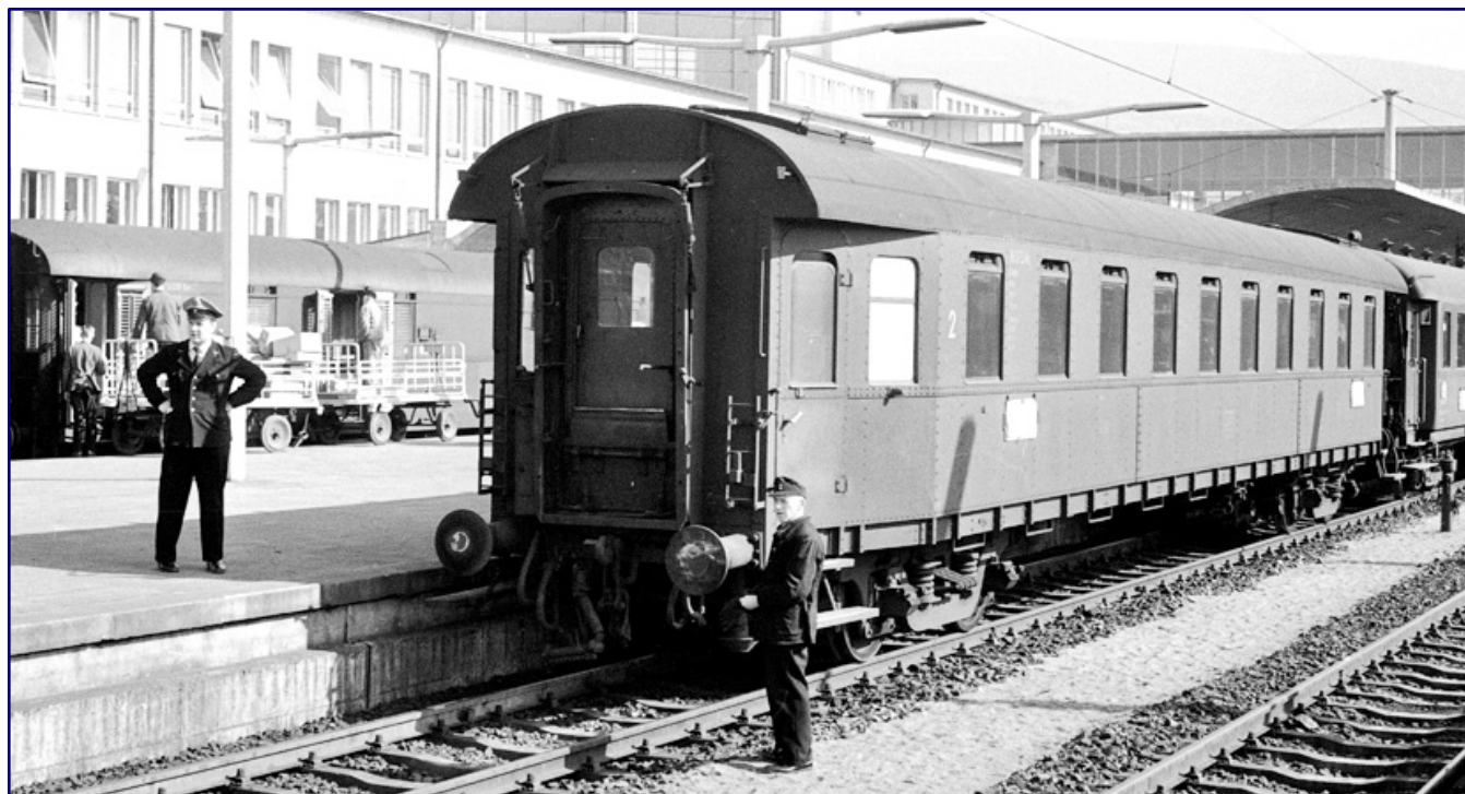
The C4ü-26 (type 1926) ran on swan-neck bogies with a wheelbase of only 2,150 mm. The carriage ends still corresponded to the Hech wagons (1921 - 1923 design), while a continuous barrel roof was already being used. This marked the transition to the 1928 to 1930 design. Photo: Karl Friedrich Walbrach | Eisenbahnstiftung
