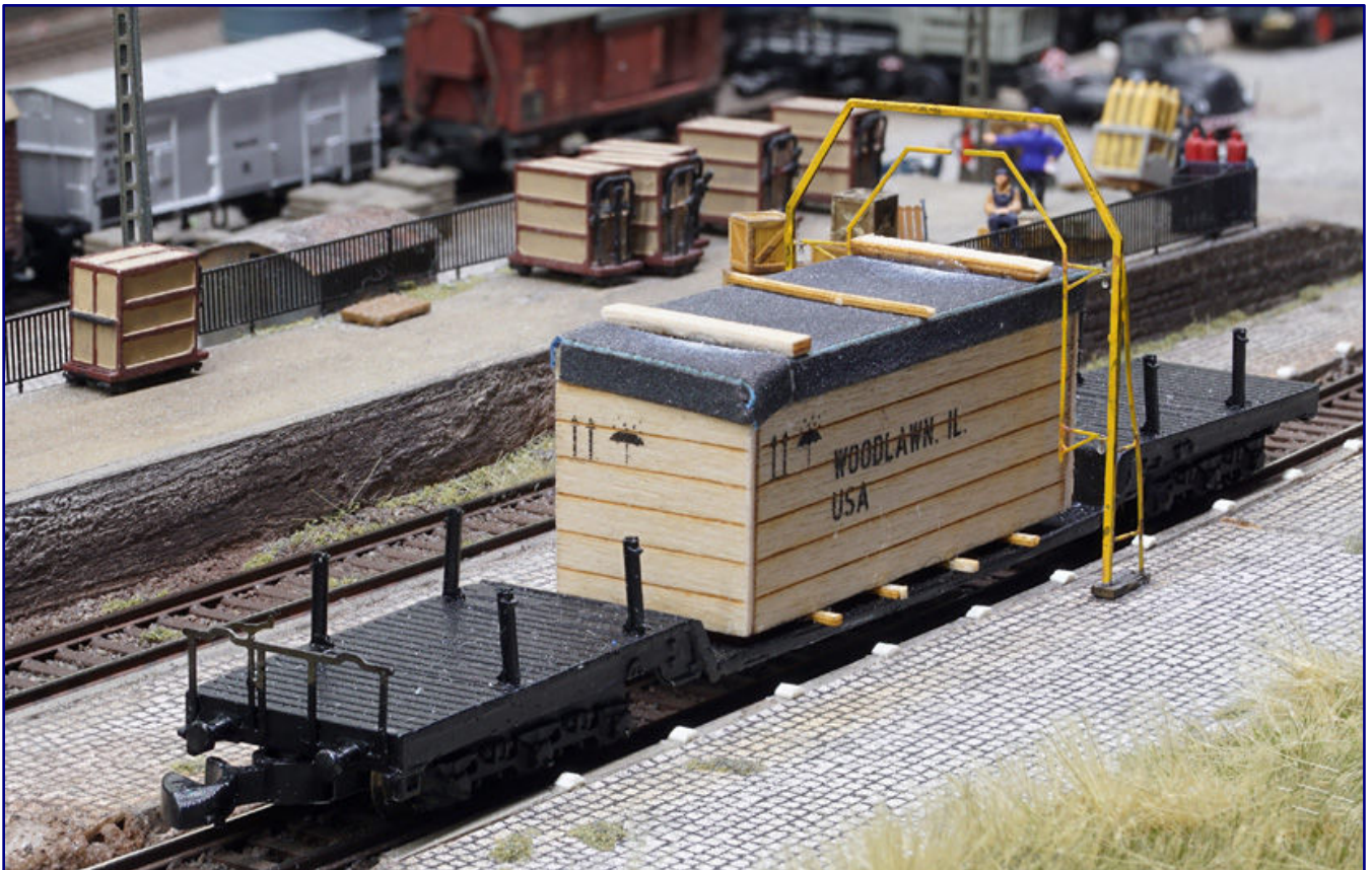
The wagon fits through the loading gauge perimeter profile with the machine box loaded. It can therefore be used in regular goods trains and travels without any special precautions.
