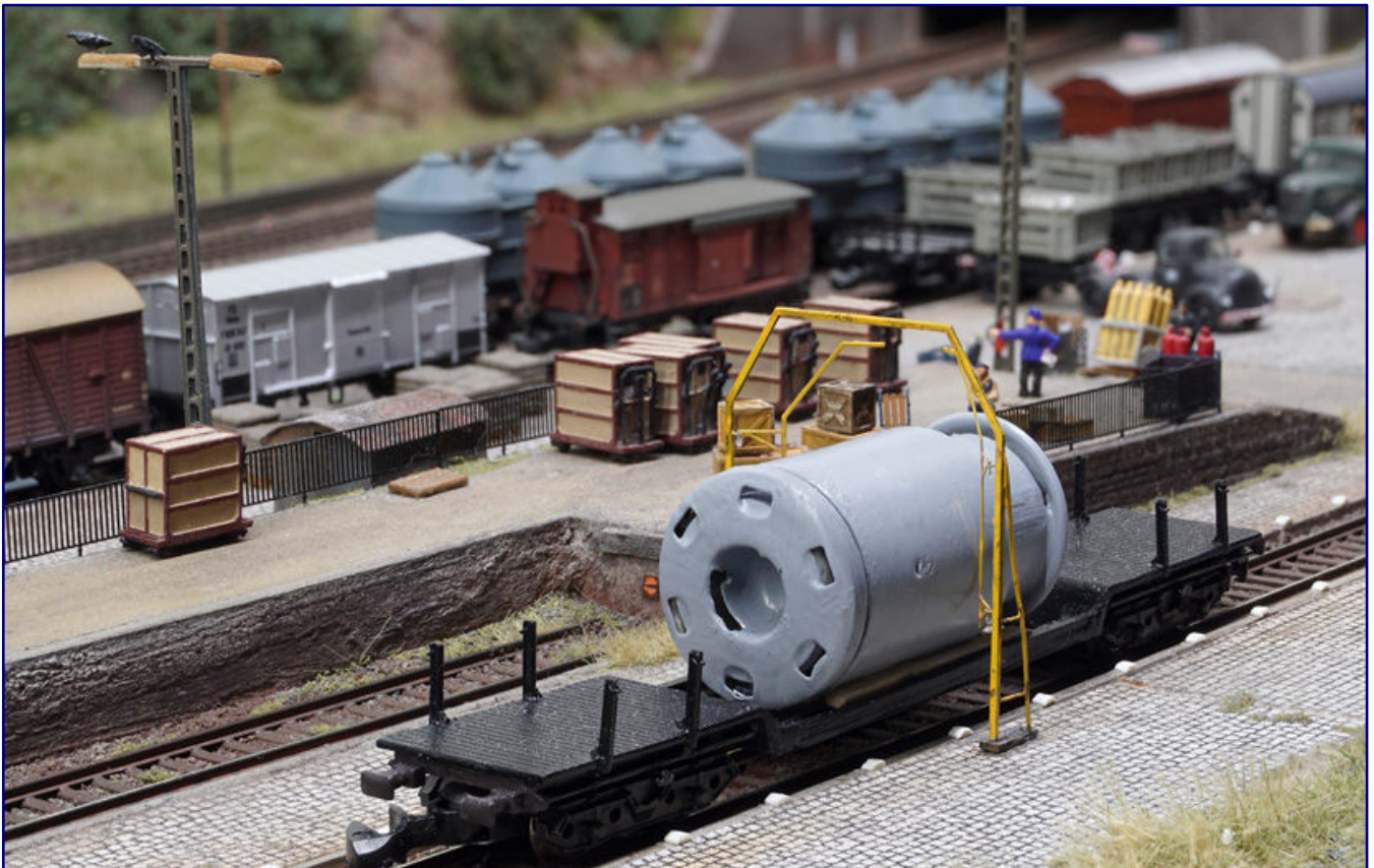
A sliding wall railcar with bogies was sacrificed for the SSt 36 and fitted with polystyrene profiles (photo above). The load was made from plastic pipe and the remains of a push button (centre photo). When passing through, the loading gauge just folds away (bottom photo), which requires transport as “Lü Anton”.
