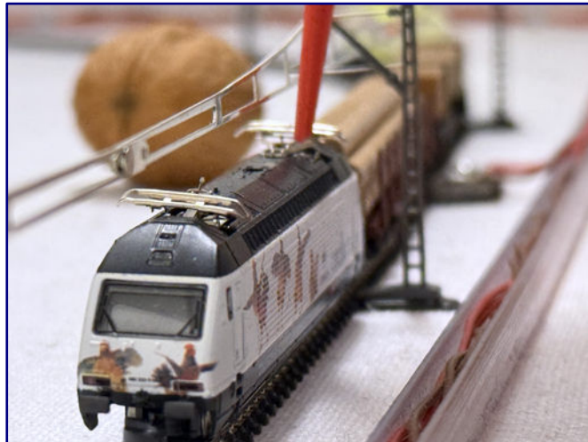
The Relax locomotive operates from the catenary wire with its pantograph and is electrically powered via this (top picture), as can be seen from the headlights. If the pantograph is pushed down (right photo), the headlights turn off.
