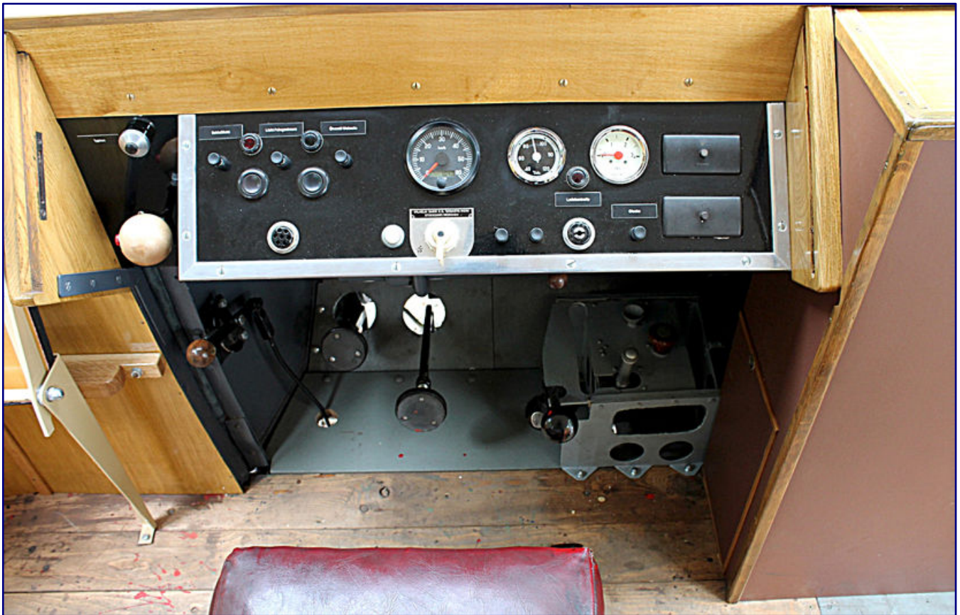
The upgraded driver's cab of a Wismar railbus built in 1933 with gearstick and foot pedals clearly shows that it is technically just a bus on rails. Photo: Jacek79 (CC-BY-3.0)
